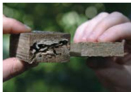
Untreated wood (left), LP SmartSide (right)
